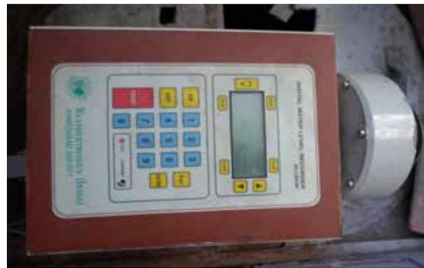
**FIGURE 7.1: A DATA LOGGER AND SHAFT ENCODER AS AN INTEGRAL UNIT**
