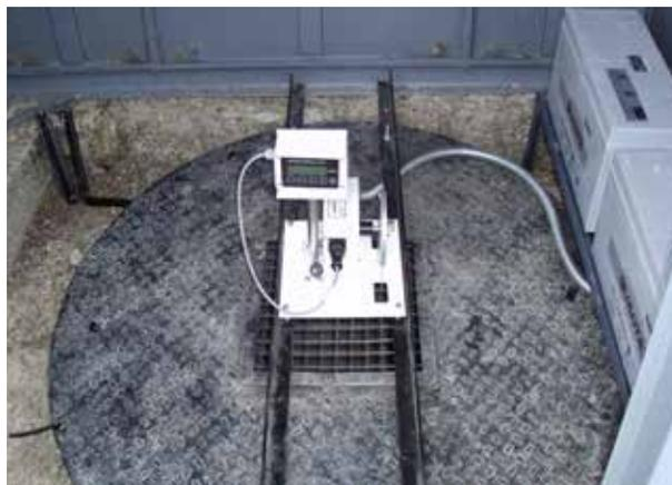
**FIGURE 3.10A:** AN EXAMPLE OF A SHAFT ENCODER INSTALLED IN MAHARASHTRA
