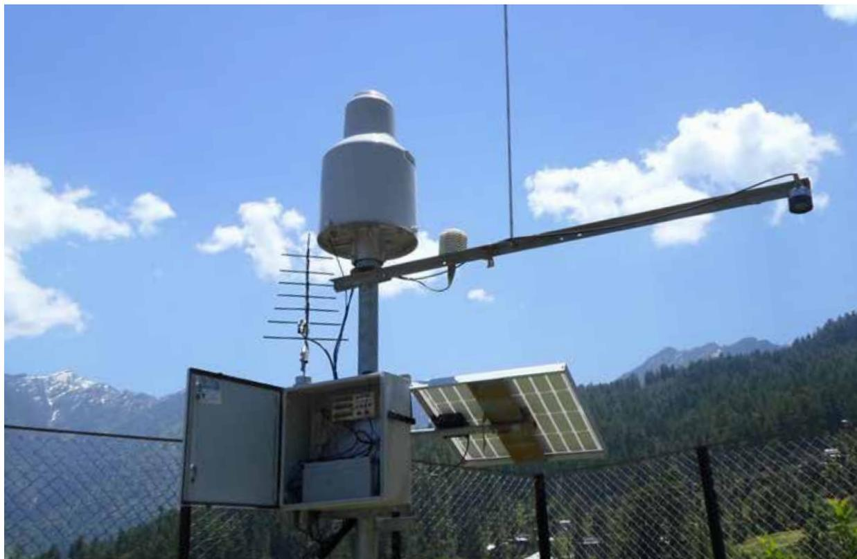
**FIGURE 2.4: A PRECIPITATION GAUGE INSTALLED IN MADANA, HIMACHAL PRADESH, BY THE BHAKRA BEAS MANAGEMENT BOARD**
