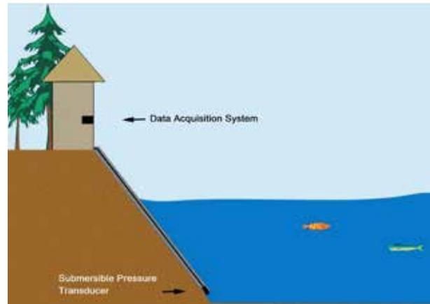
**FIGURE 3.13: A SUBMERSIBLE PRESSURE TRANSDUCER INSTALLATION**
