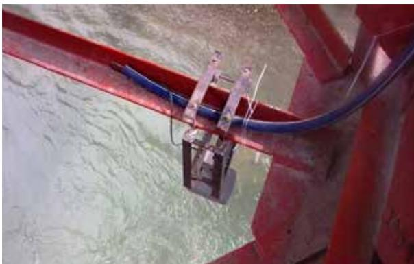
**FIGURE 3.8: A RADAR SENSOR INSTALLED ON A BRIDGE AT SAINJ IN HIMACHAL PRADESH BY THE BHAKRA BEAS MANAGEMENT BOARD**
