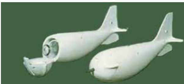
**FIGURE 6.3: A DEPTH-INTEGRATING SUSPENDED SEDIMENT SAMPLER**
