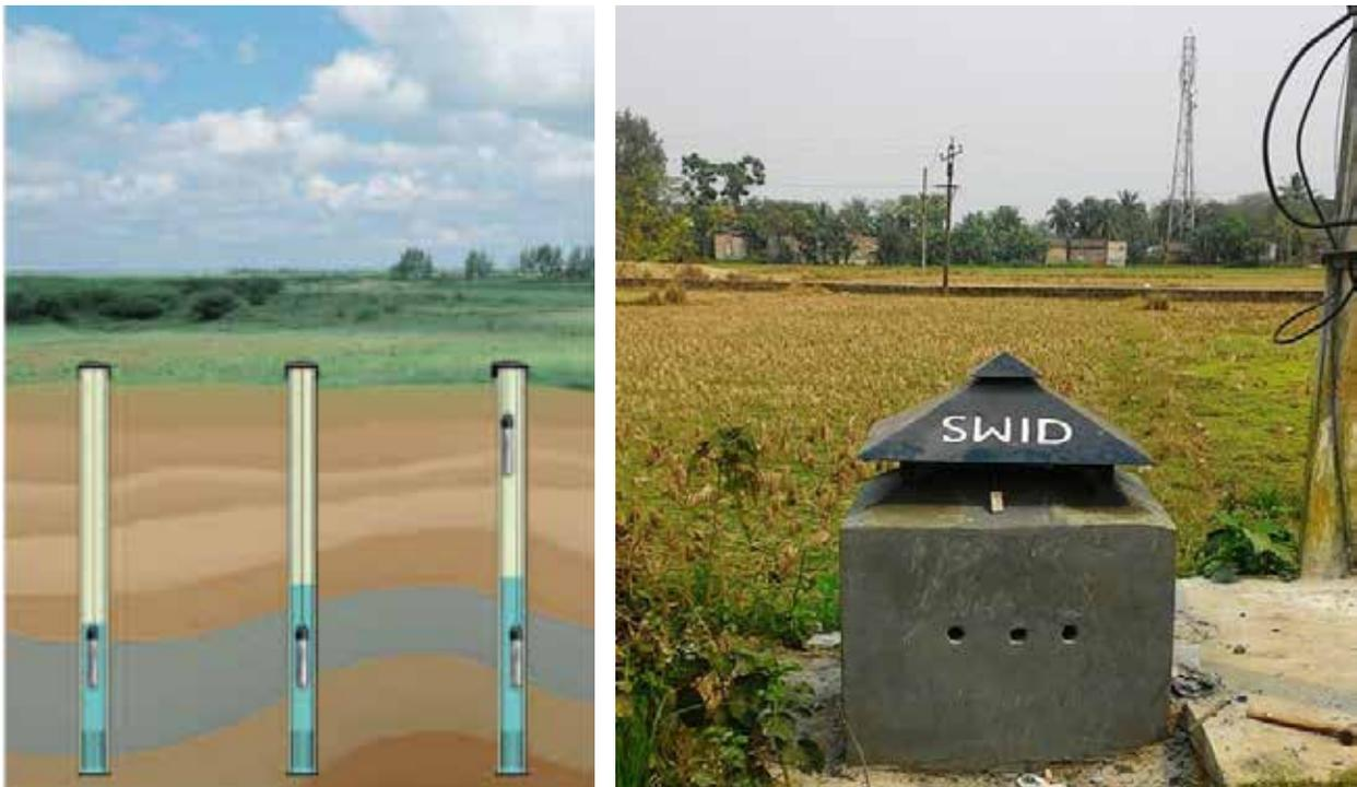
**FIGURE 4.1: A) WATER LEVEL RECORDERS INSTALLED IN MULTIPLE AQUIFERS (LEFT); B) THE SECURED STRUCTURE FOR TELEMETRY DESIGNED BY THE STATE WATER INVESTIGATION DIRECTORATE, GOVERNMENT OF WEST BENGAL (RIGHT)**
