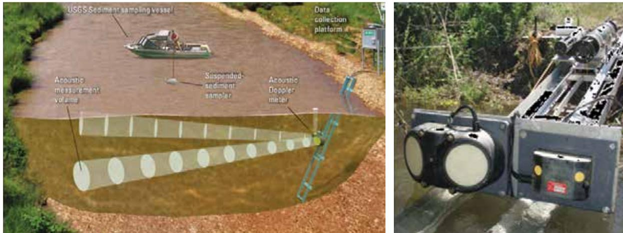
**FIGURE 6.6: AN ILLUSTRATION SHOWING THE USE OF AN ACOUSTIC DOPPLER VELOCITY METER IN CONJUNCTION WITH A SUSPENDED SEDIMENT SAMPLER FOR CONTINUOUS MONITORING OF SUSPENDED-SEDIMENT CONCENTRATION**
