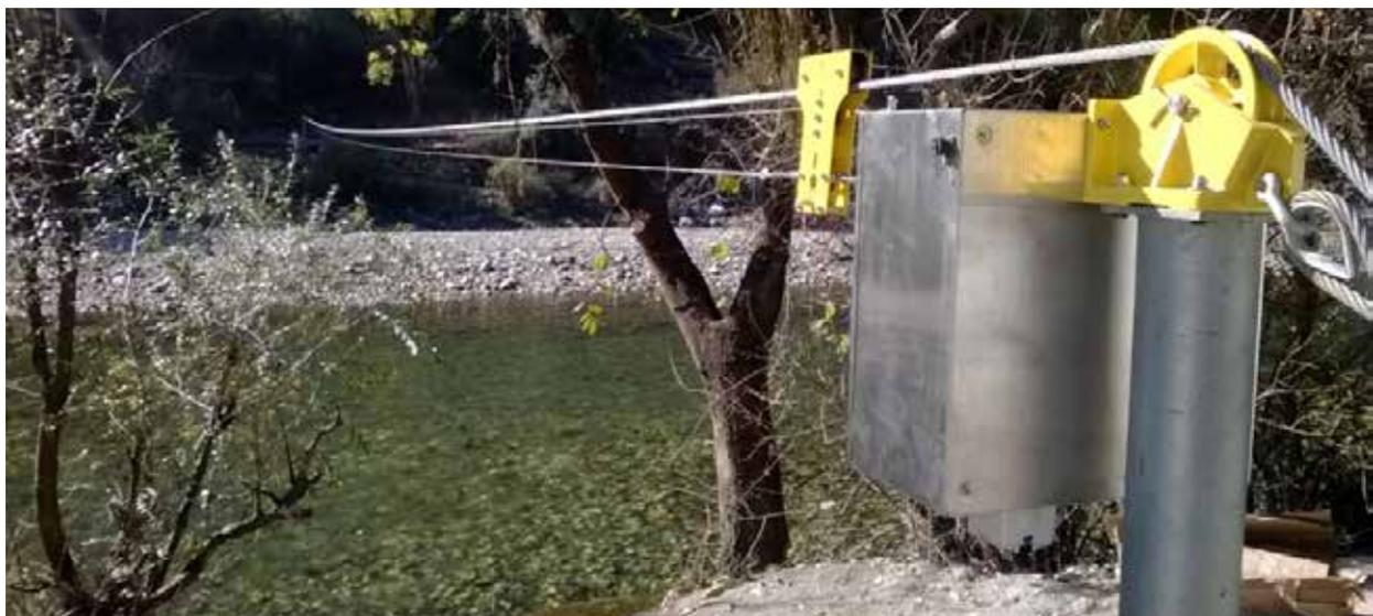
FIGURE 3.23 (A): AN AUTOMATIC CABLEWAY INSTALLED ON BEAS RIVER IN HIMACHAL PRADESH
