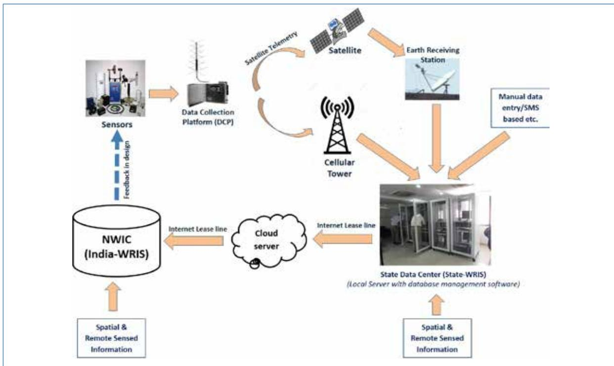
FIGURE 11.2: DATA STORAGE AND TRANSMISSION USING E-SWIS
