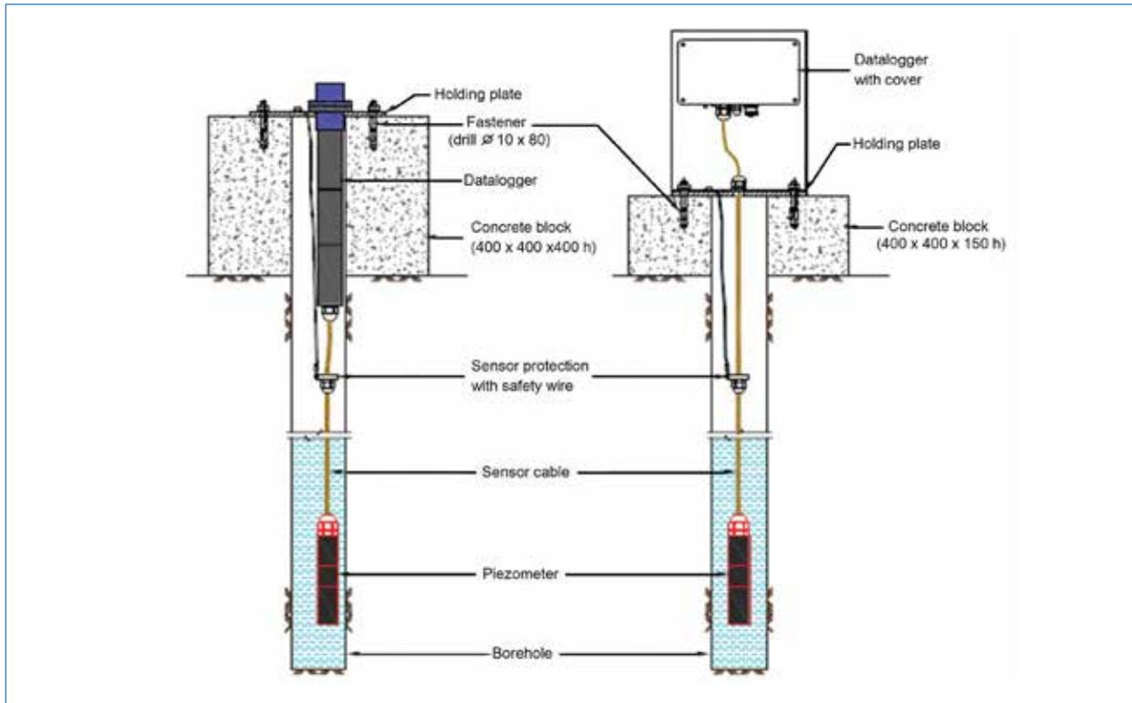
**FIGURE 4.1: C) AUTOMATIC WATER-LEVEL SENSORS WITH AN INTERNAL DATA LOGGER AND EXTERNAL DATA LOGGER FOR MULTI-PARAMETER MONITORING AND TELEMTRY**
