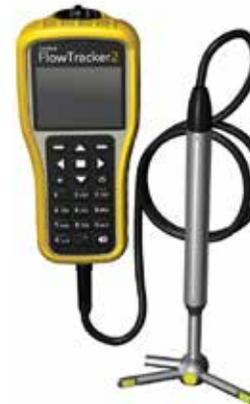
FIGURE 3.22: A HAND-HELD ACOUSTIC DOPPLER VELOCITY METER
