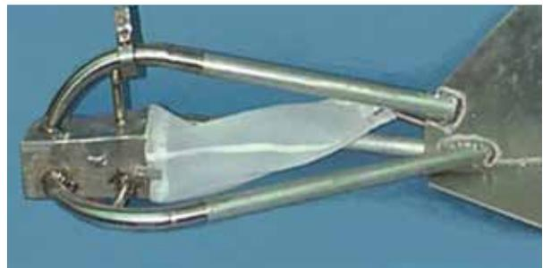
**FIGURE 6.4: HALLEY SMITH BEDLOAD SAMPLER**
