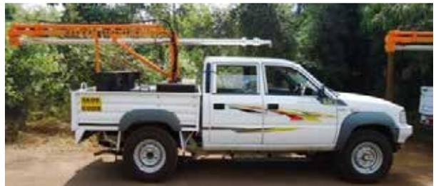
FIGURE 3.26: A VEHICLE-MOUNTED CRANE FOR DEPLOYMENT OF ADCP FROM A BRIDGE
