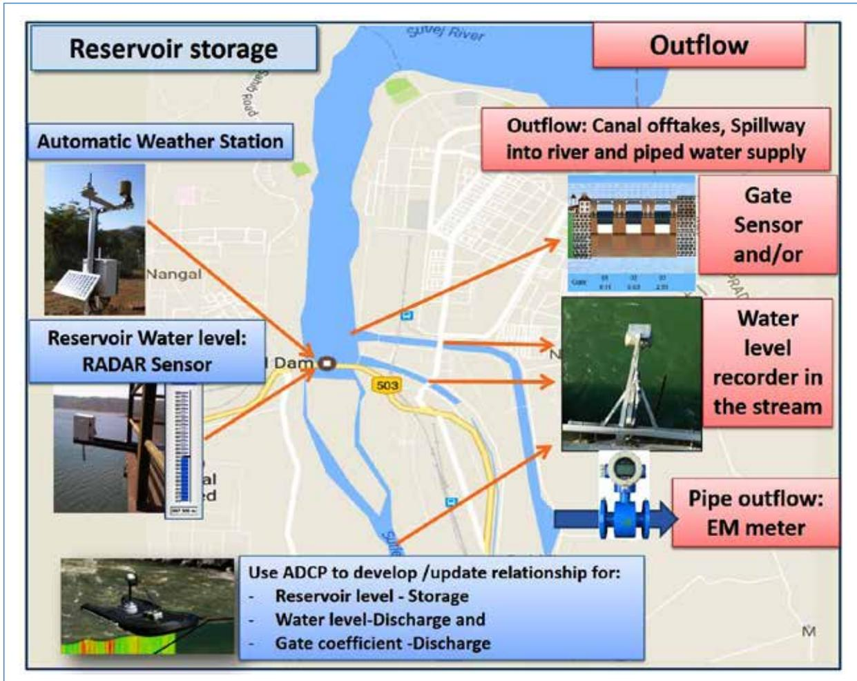
FIGURE 10.1: A TYPICAL LAYOUT FOR INTEGRATED RESERVOIR MONITORING
