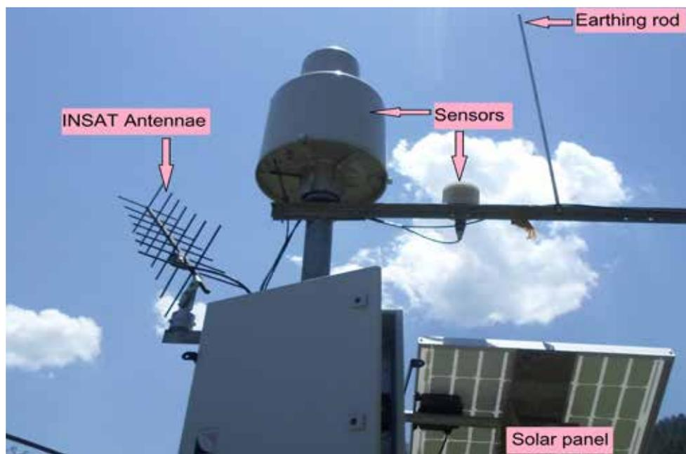
**FIGURE 7.3: EQUIPMENT INSTALLED ON THE POLE OF THE DCP**
