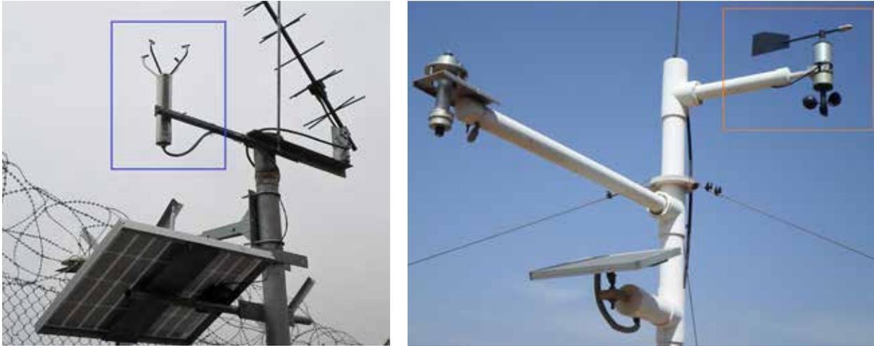
**FIGURE 2.9: AN ULTRASONIC WIND VELOCITY AND DIRECTION SENSOR (LEFT) AND A CUP-ANEMOMETER AND WIND VANE-BASED WIND VELOCITY AND DIRECTION SENSOR (RIGHT)**
