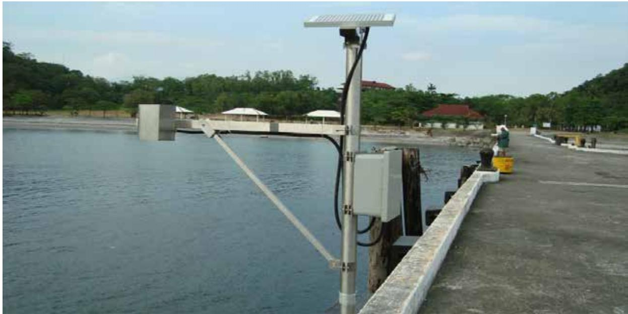
**FIGURE 3.5: AN ULTRASONIC SENSOR WITH A BOOM MOUNT**
