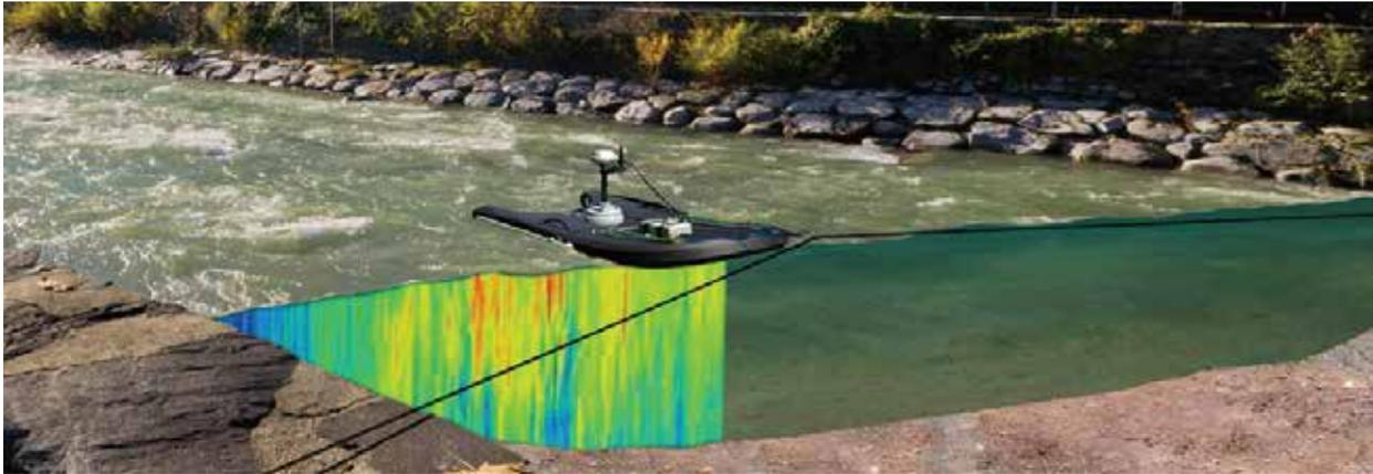
FIGURE 3.21: AN ADCP AND A TETHERED FLOAT
