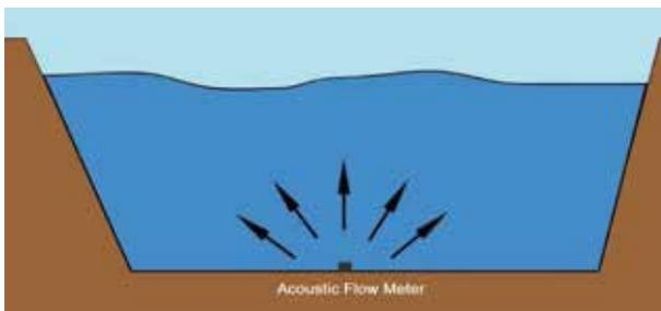
**FIGURE 3.17: THE SCHEMATIC OF AN UPWARD-LOOKING ADCP**
