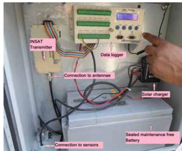
**FIGURE 7.2: EQUIPMENT INSTALLED INSIDE THE BOX ON THE DCP**
